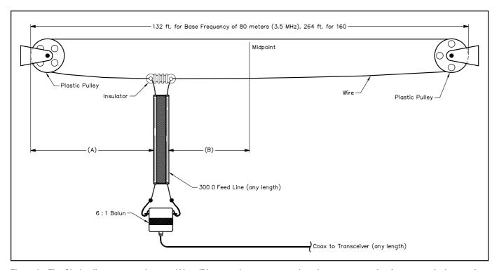
Figure 3—The Clothesline antenna. Just set (A) or (B) to equal a quarter wavelength at your operating frequency. As long as it is a multiple of your base frequency (most HF ham bands are), your antenna is tuned. You can measure out your favorite bands, peak them by observing the SWR, and put color marks or tags on the bottom wire. Roll up to the mark and you're ready to couple to the cosmos!
